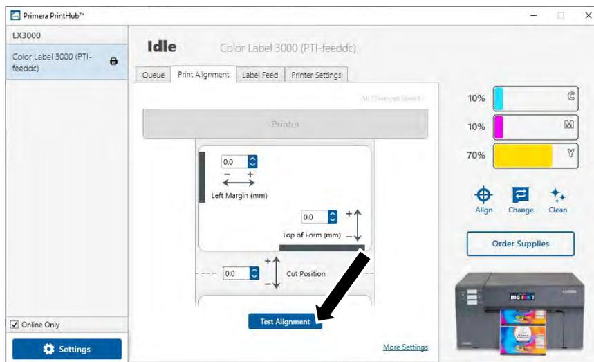
**Important!** Before adjusting any values, print the test alignment to see how close you are to alignment. The on-screen graphic is the same as the print, which makes it easier to adjust these values.
